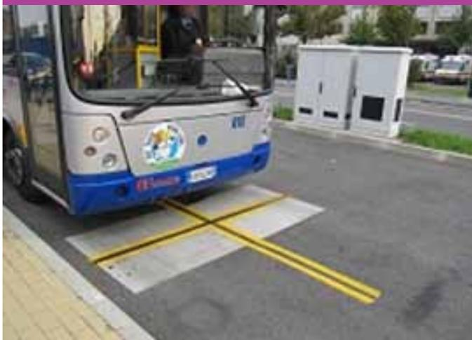
The system which was of most interest for potential application in Birmingham is one which uses the same technology used to charge phones and toothbrushes wirelessly, but used on a much larger scale. This form of induction relies on magnetic charge plates beneath roadways and a counterpart inside the vehicle. When vehicle
