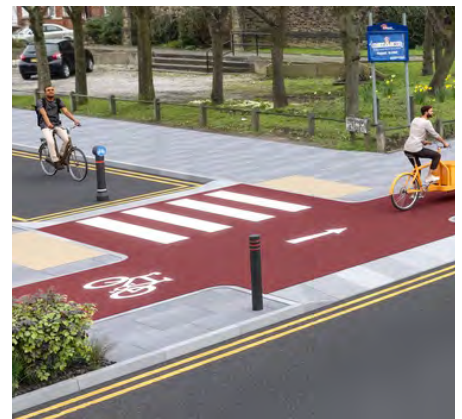
Image: Dutch entrance kerbs Credit: InfraCGI
