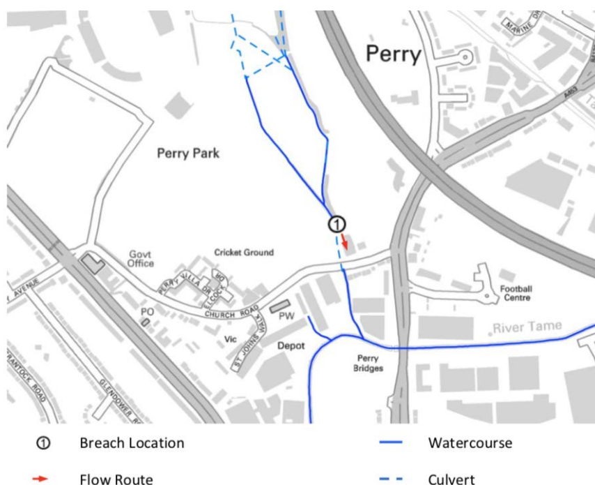
Figure 4-21 Potential watercourse breaches and overland flow routes
