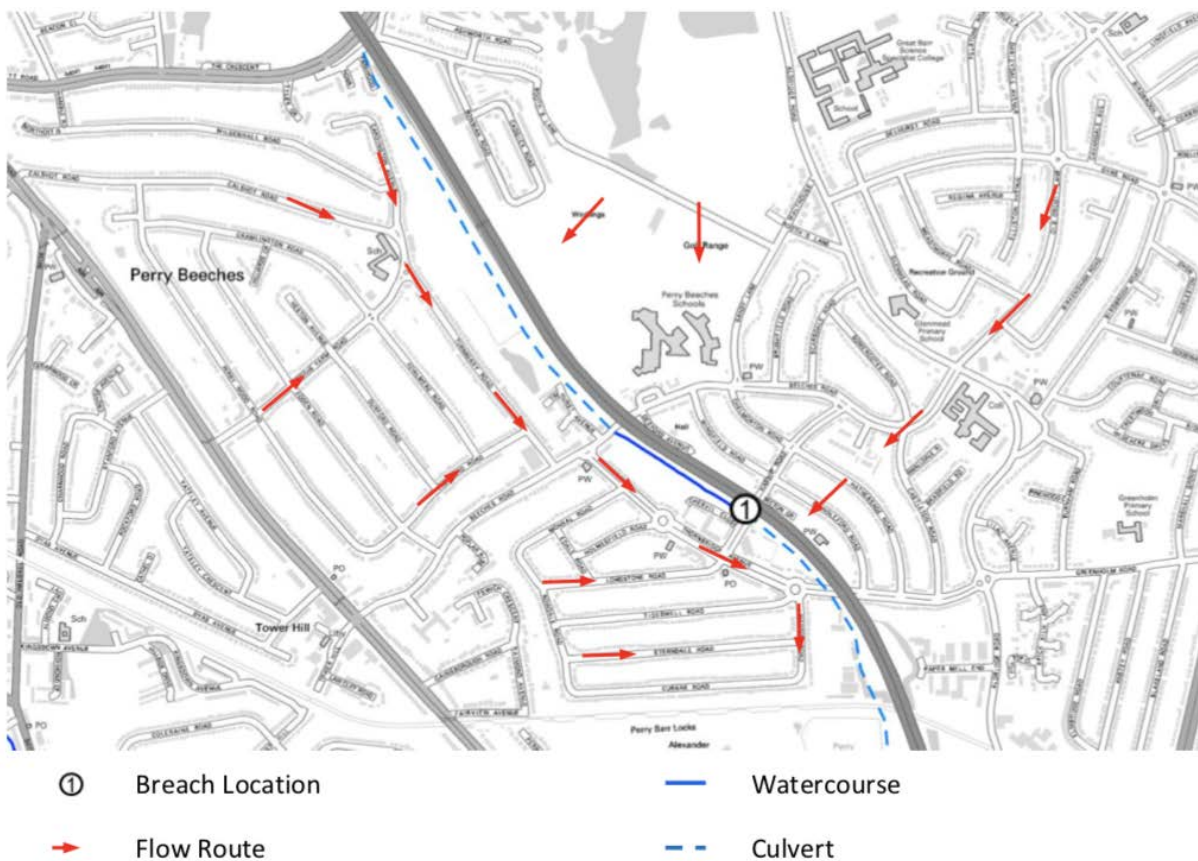
Figure 4-24 Potential watercourse breaches and flow routes
