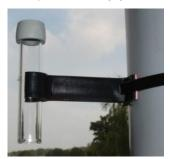
**Description:** Acrylic tube fitted with coloured and white thermoplastic rubber caps. The coloured cap contains the absorbent.
