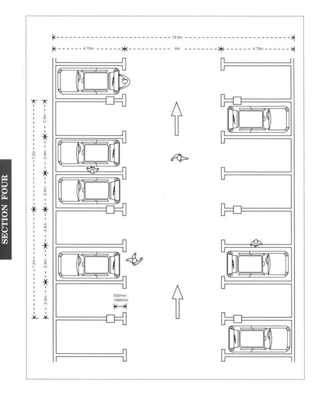
Figure 13: Illustrates the dimensions of spaces and aisles for 90 degree parking
