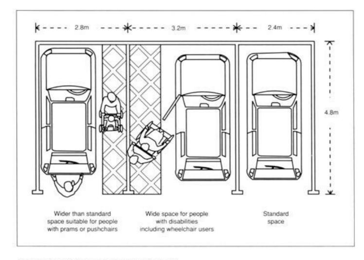
Aisles should have a minimum width of:
