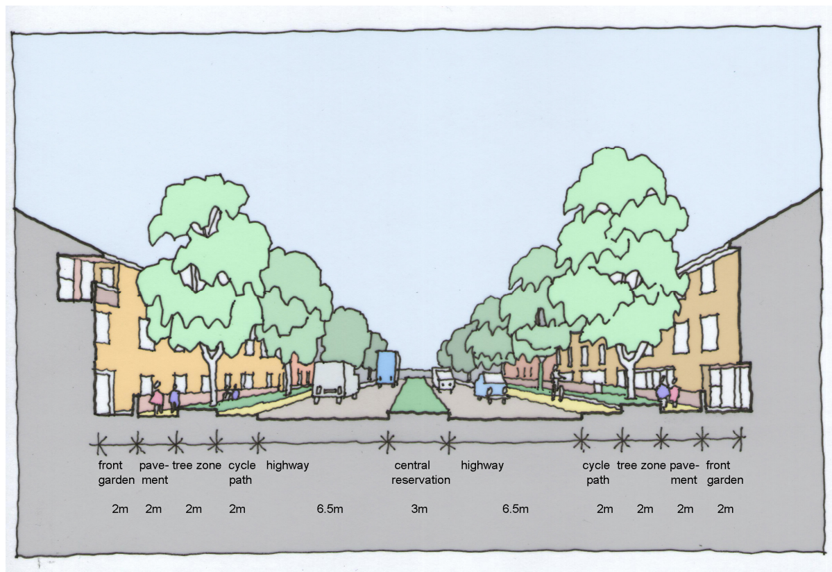
Fig 3B: Highgate Road housing site: illustrative cross section
