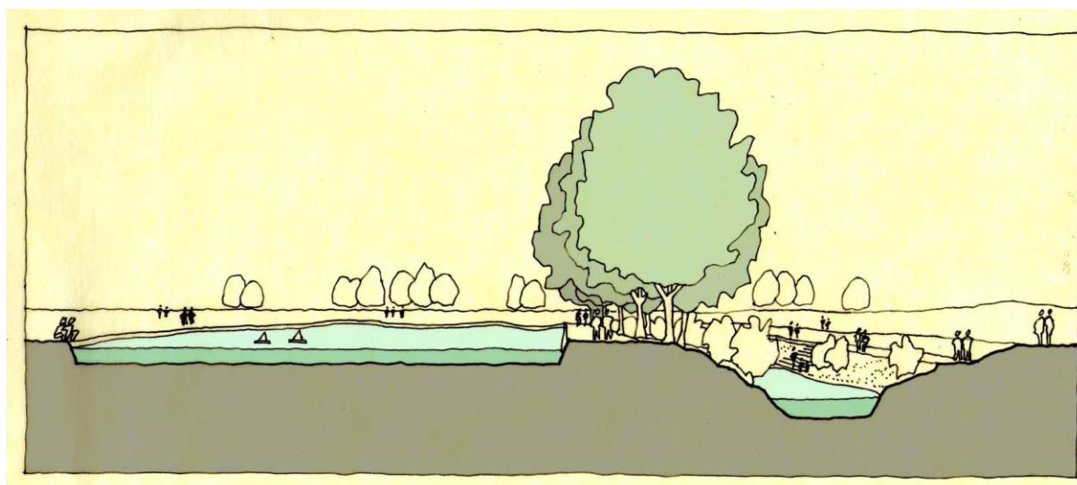
Fig 5: River Rea naturalisation: illustrative cross-section
